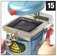
...raise the orange handle to lower the softened plastic onto the pattern.
