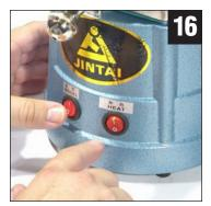
After about 8 seconds (to allow the plastic to cool), turn off the vacuum.
