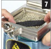
Use your fingers to push the metal beads around the bottom perimeter of your pattern. This will keep the plastic from wrapping around the pattern, making it difficult to remove later in the process.
