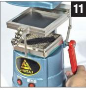
Push the orange handle down to latch the metal frame in the UP position.
