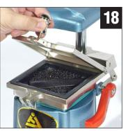
Unlock the frame and swing up the top half.
