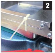
Use diagonal cutters or a knife to snip the cable tie holding the frame parts during shipment.
