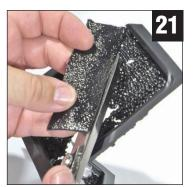
Cut excess plastic sheet from the vacuum formed part.
