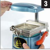
Rotate the heater all the way to the left to get it out of the way for the next few steps.
