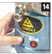
Moving quickly, turn off the Heat. Then, turn on the vacuum using the "Model" switch, and...
