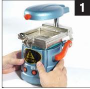
Unpack the machine and place it on your workbench in the position shown. Notice that the orange handle is in the horizontal position and the two control switches on the front of the machine are in the OFF position. Plug the line cord into a wall outlet. Note: The heater draws a lot of current, so try to avoid using an extension cord that could overheat.
