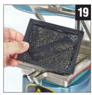
Remove the plastic sheet from the vacuum chamber. Watch out for all the metal beads that may stick to the plastic. Pop them out over a large tray or pan to catch them for re-use.
