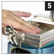
Use your fingers to spread out the metal beads evenly in the vacuum chamber.
