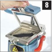
Swing up the top half of the frame. It should stay in place.
