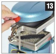
Grab the heater knob (do not touch the metal part of the machine – it gets HOT!). Swing the heater over the center of the plastic sheet and watch for the plastic to soften and sag down in the frame about <sup>3</sup>/<sub>4</sub>". Experiment with different amounts of sag for different plastics; your experience will help judge when to do the next step.
